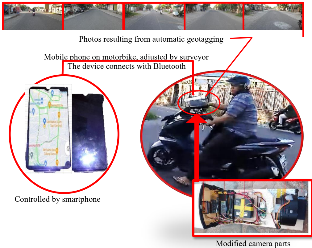
Fig. 2. A set of road condition survey equipment.
