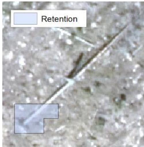
Fig. 5. Commission error caused by trees fell between LiDAR data and orthophoto images.
