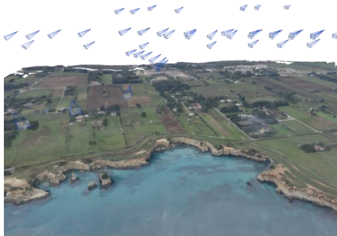
Fig. 7. Screenshot of the 3D point cloud and camera poses.
