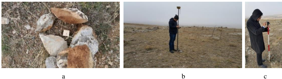
Fig. 9. View of used wooden pile (a); view of measurement with Topcon Hiper V GNSS Receiver (b); View of measurement with Asus Zenfone 6 using Kocaman Pro Software (c).
