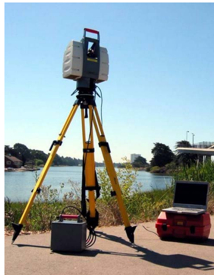
Fig. 6: In the field with Leica HDS ScanStation
