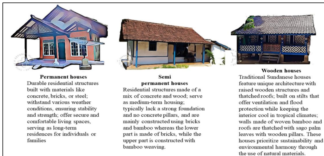
Fig. 6. The type of the houses in the area, nearly all of the permanent houses in the area do not meet the standard for earthquake resistance.
