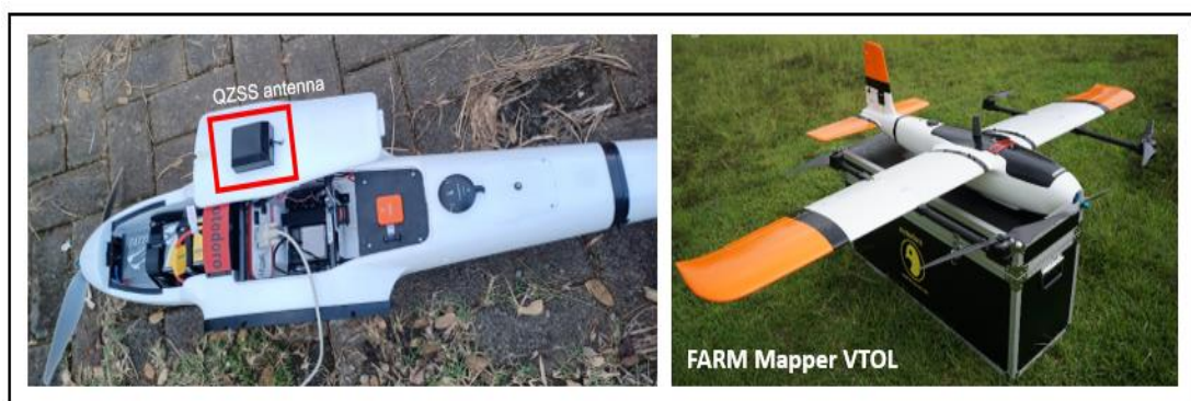
Fig. 2. QZSS antenna installation on Fixed-wing UAV.
