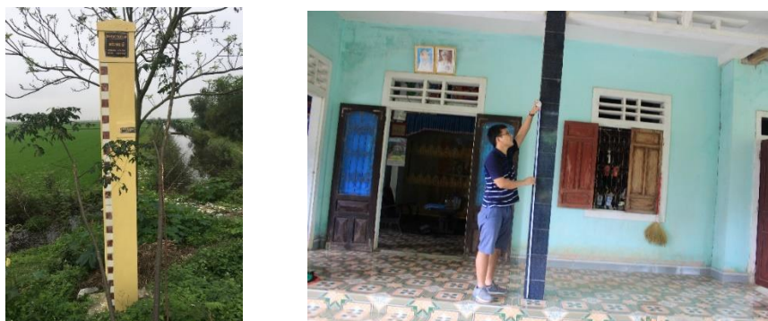
Fig. 2. – The flood marks in the Nhat Le – Kien Giang in 2020 (left) and 2013 (right). These flood marks were recorded by GPS with X and Y coordinates in 2015 and 2022 in Hong Thuy commune – Le Thuy district, Quang Binh, Vietnam. These are two historic floods in Vietnam, have significant effects on human life and the country's economy. Source: Huu Duy Nguyen 2022 and 2015.
