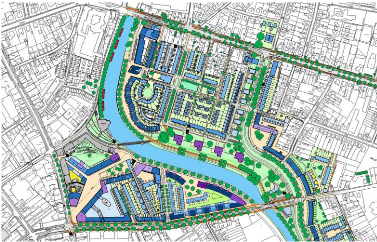
Fig. 8: Plan to renew the district of 'Kanaaloevers' in the Dutch city of 'Apeldoorn', 2008. The base map, basically cadastral and sub-divisory, is drawn using fine lines and in the range of greys (Apeldoorn Town Hall, 2008).
