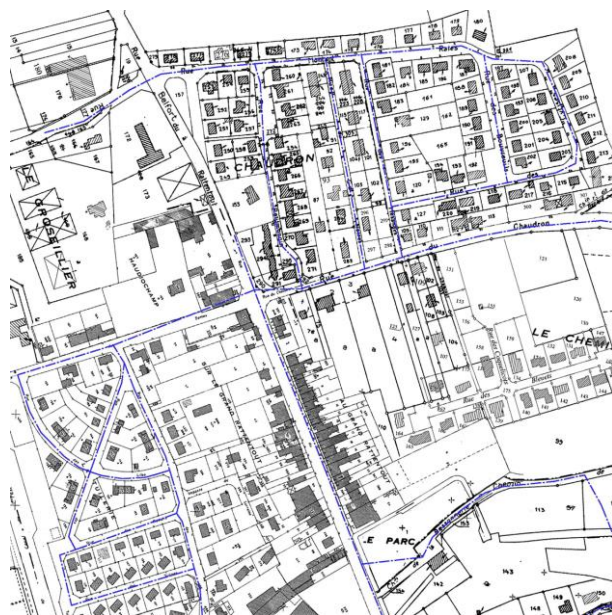
Fig. 7 Part of the plan of the main drinking water network in the town of "Dieu-sur-Mer" 6 –France- dated 2007 (ESpace & TERritoires, 2007).
