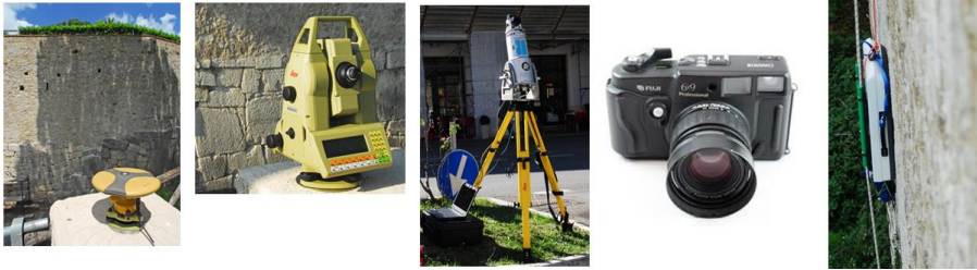
Fig. 11 Deformation monitoring techniques used.
