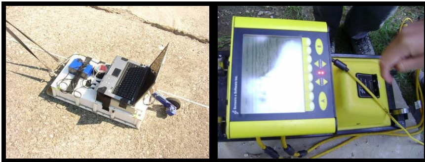
Fig. 5 GPR instruments: the Zond-e 12 GPR with a notebook on it (left), and the central unit of PULSEKKO
